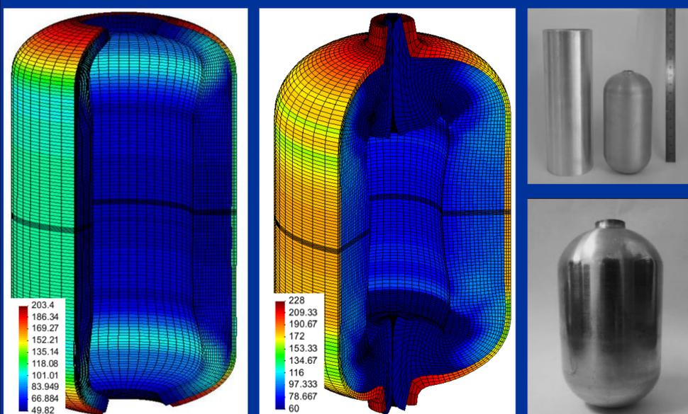
Finite element predicted distribution of effective stress (MPa) after 45 mm and 90 mm displacement of the upper die.
